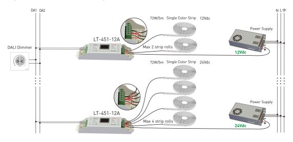
Providing DALI to 0-10V connect port, which is compatible to control 0-10V products in DALI control system, diagram example as below:
